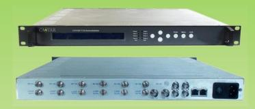
normal demodulator, this demodulator has 2 ASI inputs, supports 6 tuner inputs (DVB/C/S/S2/T) optional, two separate ASI output ports and one DATA port for two separate megabit IP outputs.
